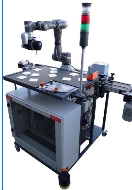
ON10: "Collaborative 2D Unscrambler & Screwdriver" in ErmaSmart Assembly configuration
