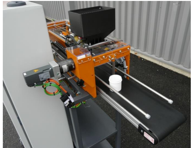
Dosaxe operating part with Module for dosing granules into pots/flasks
