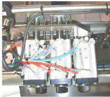
Double cleat cylinder "Entry and exit of screwing lock" + Cylinder "Indexing containing To screwing lock" + Cylinder "Clamping to screwing post".
