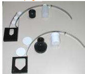
Cap dispensing magazine with screwing head for caps and containers in "bottle" format
