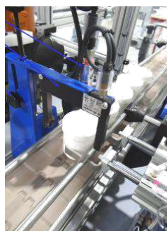
Control by presence detector cap and fork screwdriver control
