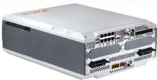
View of the KRC5 Micro controller on the robot
