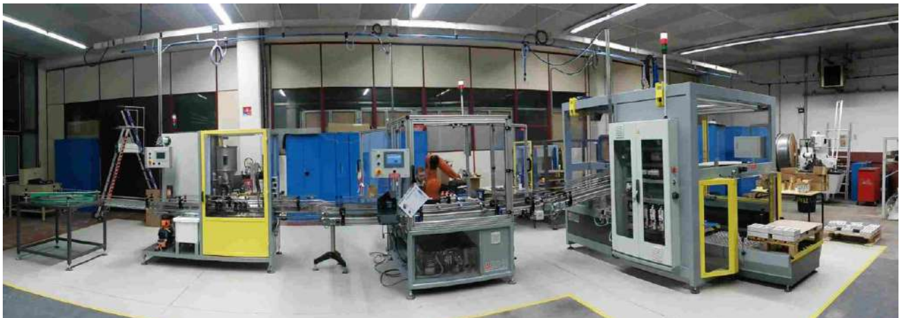
Robotic cell integrated into the Ermaflex line
