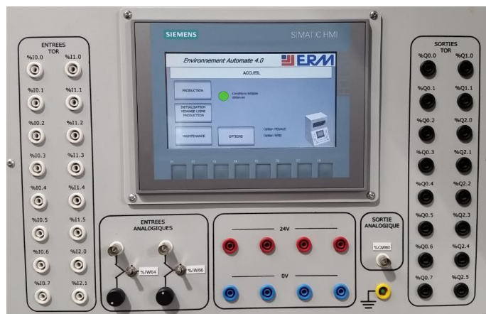
Connection interface with double-well plugs (barana plugs) and BNC connectors. And optional touch screen.
