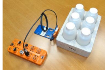
IO-Link master and RFID read-write head
