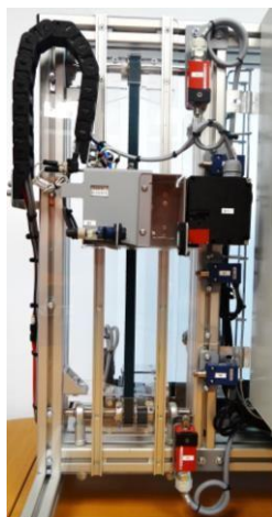
Operating part with safety and interlocking safety switches
