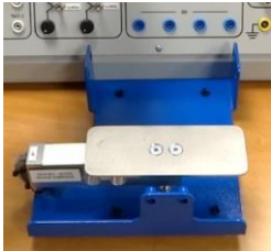
Strain gauge on the weighing station
