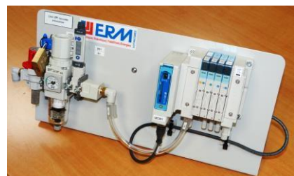
Pneumatic valve assembly with IO-Link communicating pneumatic island and pressure switch
