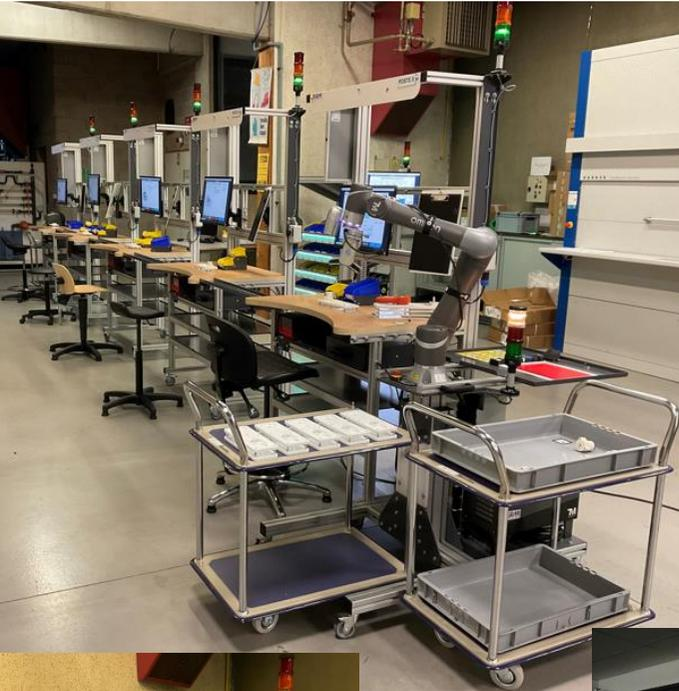
*ErmaLean in right configuration, with Omron TM5 Cobot & Vision Station*
