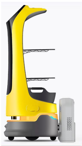
Automatic charging station
