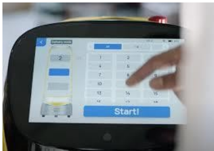
Touch panel for interact with the robot and plan the tasks to be carried out
